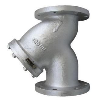
**UNIMAC Strainer** are available in Angle & 'Y' type , and are available in Cast Iron ,Cast Steel, MS Fabricated, Flange type, provided with filter element. Filter element is made from Brass/ Bronze/ Stainless Steel having standard 40 mesh and supported with perforated sheet. Sizes available from 15 mm to 500 mm and strainers are tested at required pressure at our works prior to despatch.
