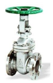
UNIMAC Gate Valves are provided with properly machined and lapped backseat to ensure re-packing under pressure while fully open.
