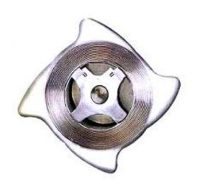
Disc Check Valves must be fitted in accordance with the direction of flow arrow indicating correct fluid flow direction. When fitted with a spring they can be installed in any place. When supplied without a spring these must be fitted in a vertical flow line with the flow from bottom to top.
